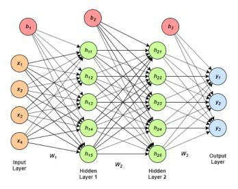
Figure 2.1: Example of a MLP with two hidden layers.
