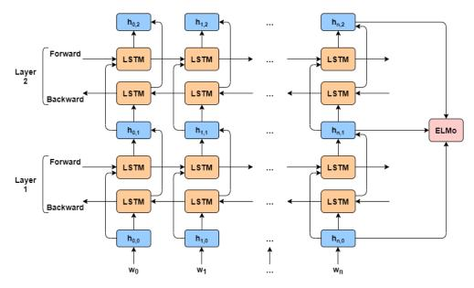
Figure 2.5: ELMo architecture for two layers.
