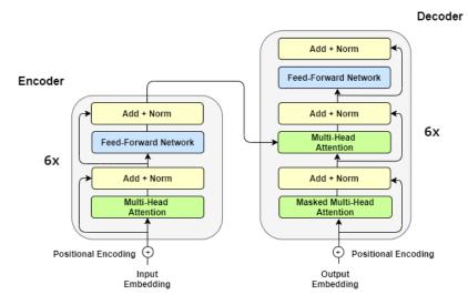
Figure 2.4: Transformer architecture.
