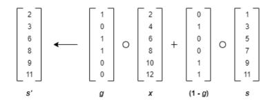
**Figure 2.3:** Example of using a binary gate vector *g* to update a state *s*.
